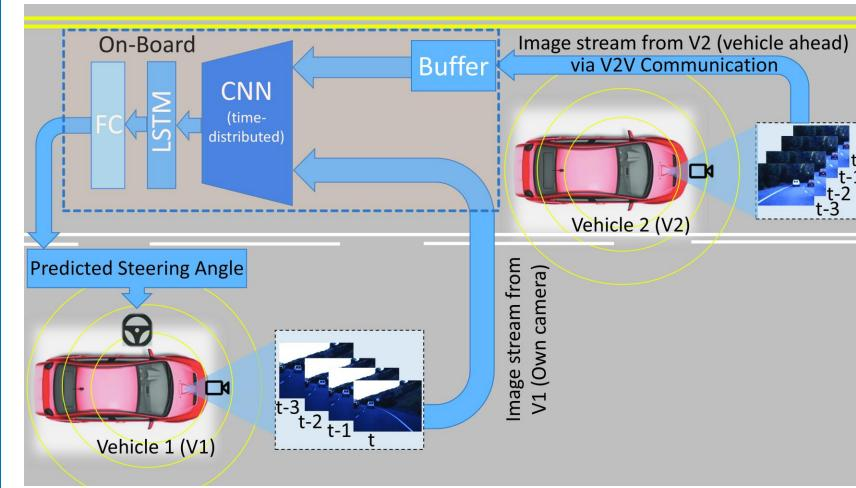
The overview of our proposed vehicle-assisted end-to-end system is given above:
